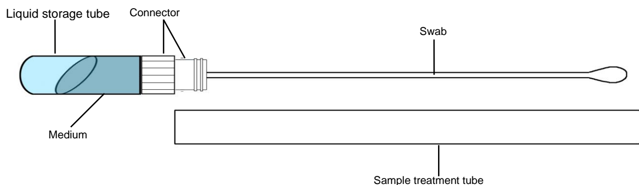
Illus 2: Structure of the AmpuSafe®102-18 device
